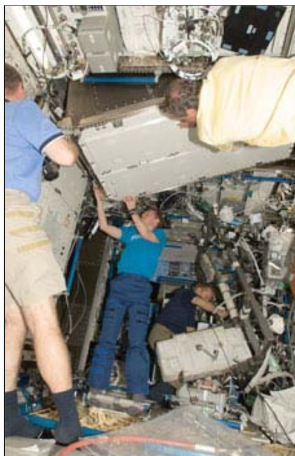
ESA astronaut Christer Fuglesang (top foreground) and NASA STS-128 astronaut Tim Kopra, install the new Minus Eighty Degree Laboratory (MELFI) Freezer on board the ISS Destiny laboratory. Credit: NASA
