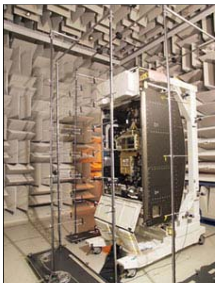
Fluid Integrated Rack/Microscopy Module is pictured during prelaunch testing in Glenn Research Center Acoustic Testing Laboratory. The system will allow the zero-g processing of fluids and examination of diverse materials in highly automated microscopy system. A Vapor Bubble heat pipe experiment was also launched with the system on Discovery. Credit: NASA
